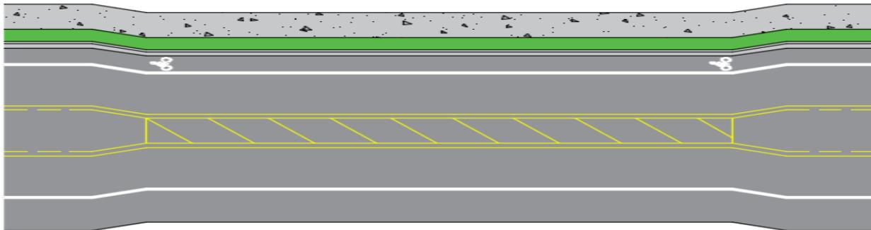
Figure 7 – Narrow median with dual lane re-alignment (not to scale)
