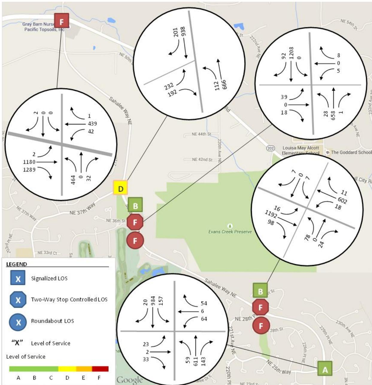
Figure 16 – 2035 Three-Lane Forecast PM Peak Hour Level of Service at Study Intersections
