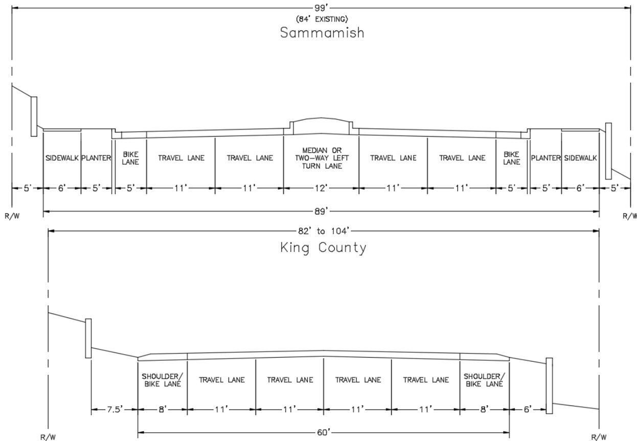
Figure 10 - Five-Lane design proposed cross sections (facing south)
