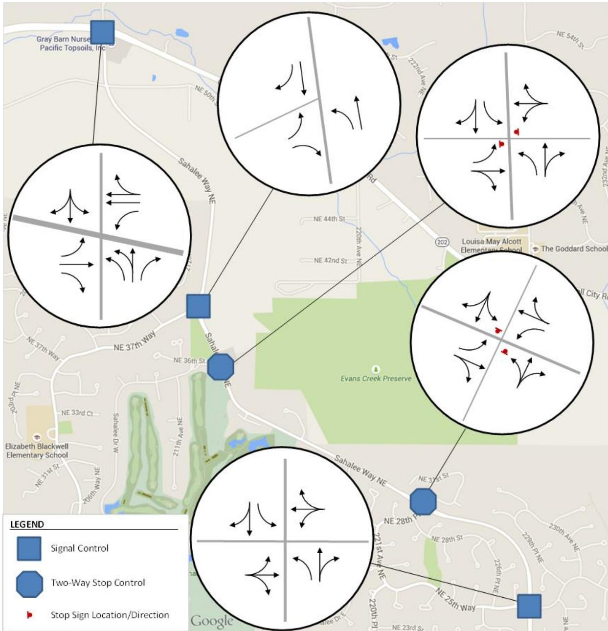
Figure 11 – Existing Lane Configuration and Traffic Control at Study Intersections
