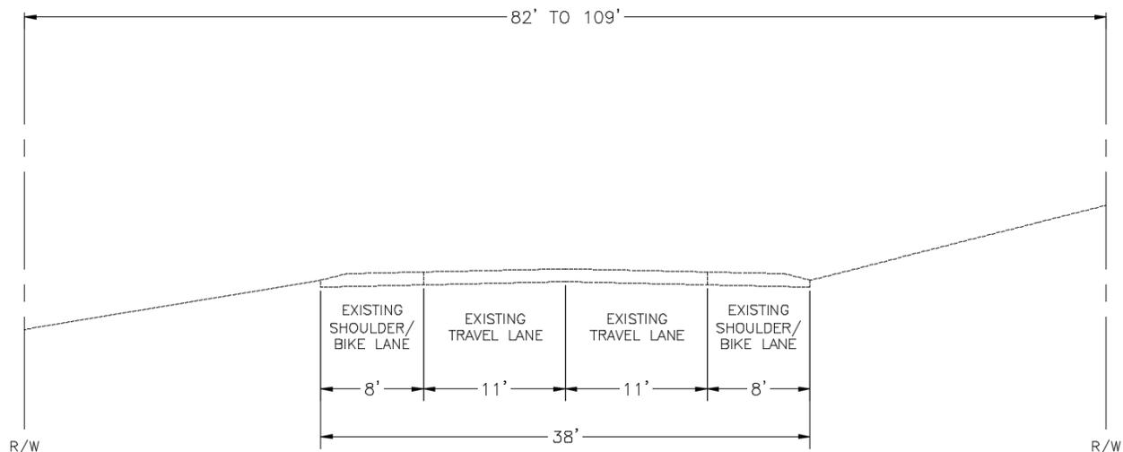
Figure 2 – Existing cross section
