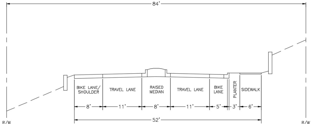
Figure 8 – Raised median island typical section (facing south)
