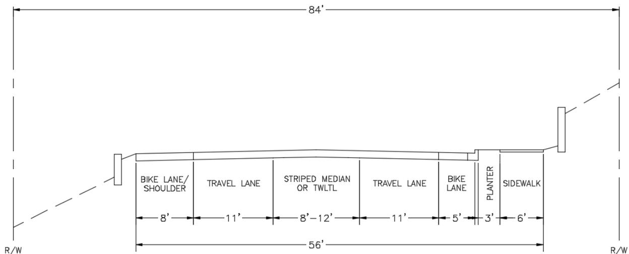
Figure 6 – Three-Lane base design proposed cross section (in Sammamish, facing south)
