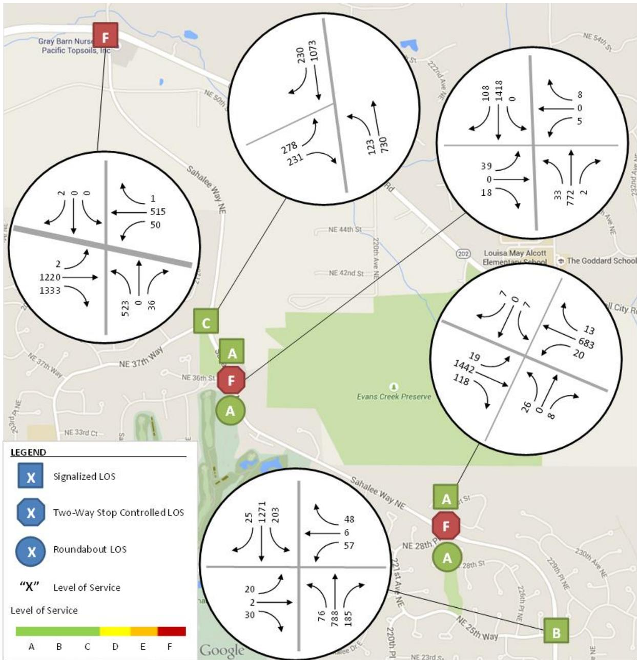
Figure 17 – 2035 Five-Lane Forecast PM Peak Hour Level of Service at Study Intersections
