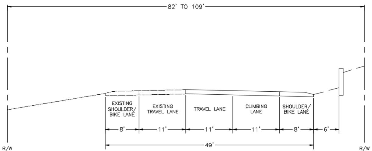
Figure 9 – Three-Lane design with truck climbing lane cross sections (facing south)
