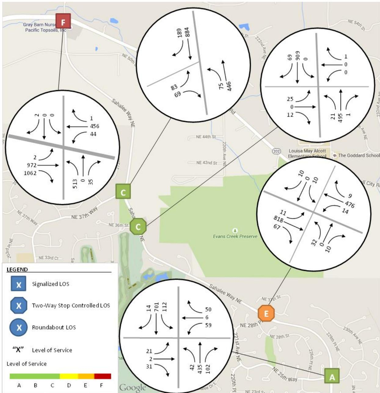
Figure 15 – 2014 Existing PM Peak Hour Level of Service at Study Intersections
