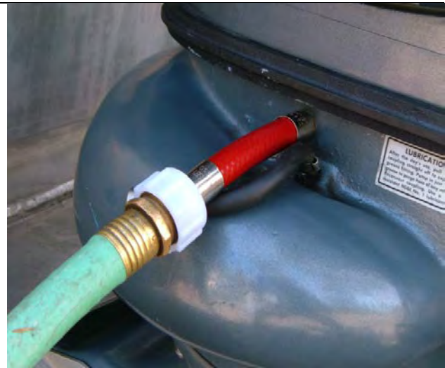
2B. Water intake bolt has been removed, and outboard flushing adapter has been attached.
