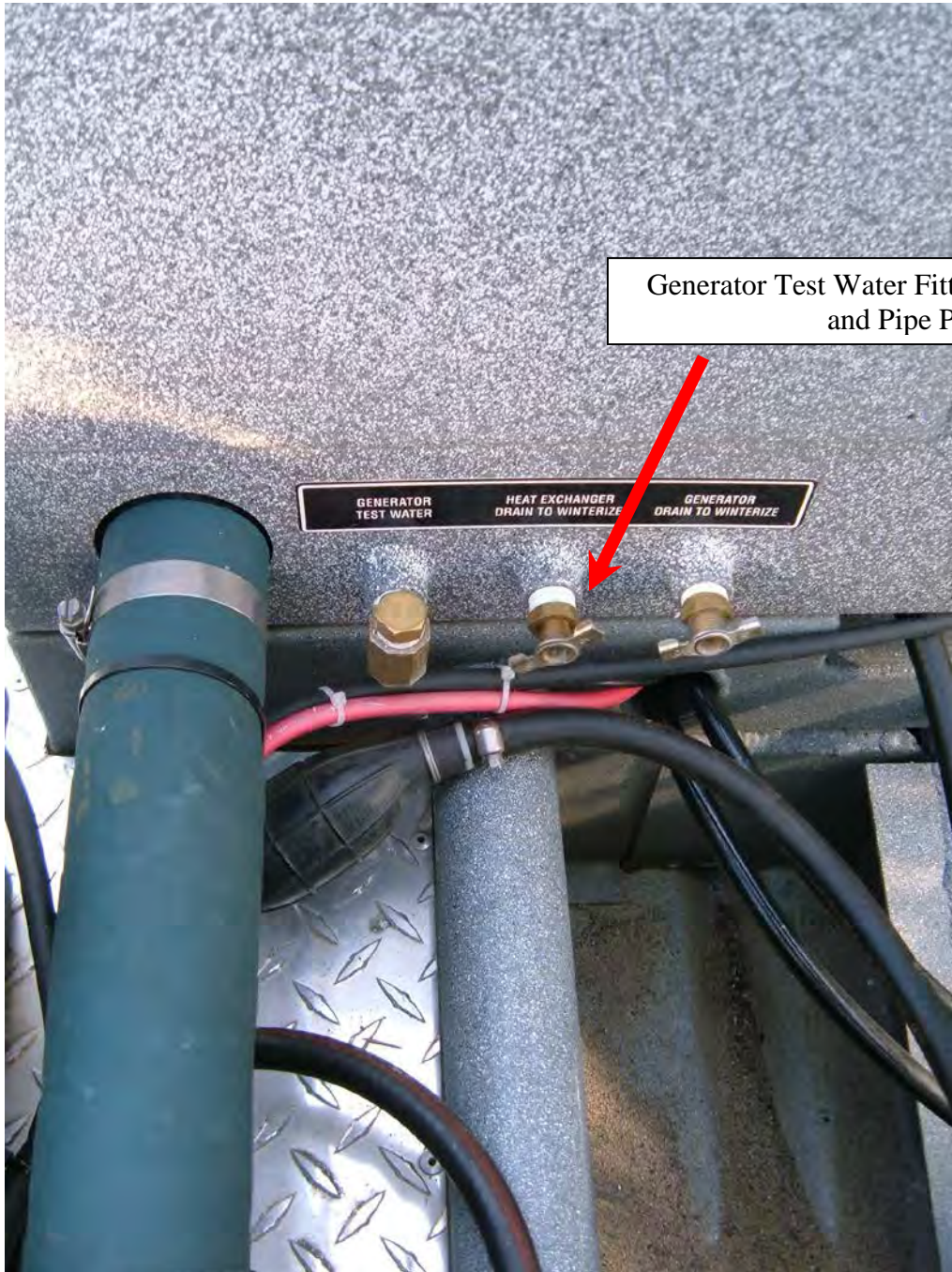
3B. Generator raw water flushing connection (i.e. Generator Test Water Fitting). Located on the base of generator cover, port side aft.
